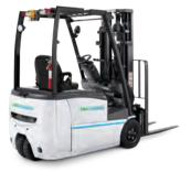
**TX-M 3-Wheel Series Cushion Tire Models** 36V / 48V Load Capacity (lbs): 3,000 / 3,500 / 4,000
