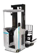
**SRX Series Reach Truck Models** 36V Single Reach Load Capacity (lbs): 3,500 / 4,500\*
